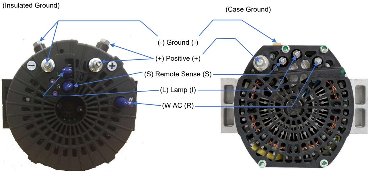
Note: Two positive and negative connections on BLD / BLP4000 series alternators are common connections. Use the connection that works best in your application.
